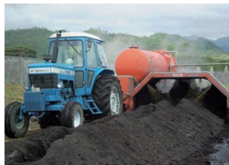
Windrow composting plant
