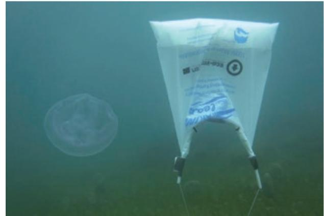
EcoOcean degradation tests in marine environment. Credit EcoCortec
