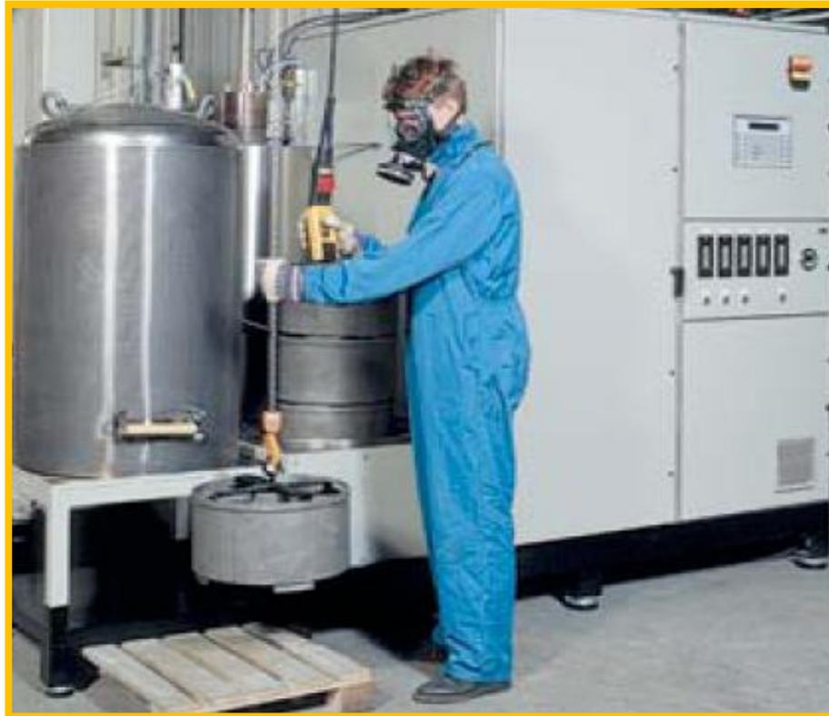
Fluorescent powders from lamps and other waste containing mercury such as button cells, dental amalgam are placed in the vacuum chamber of the distiller.
