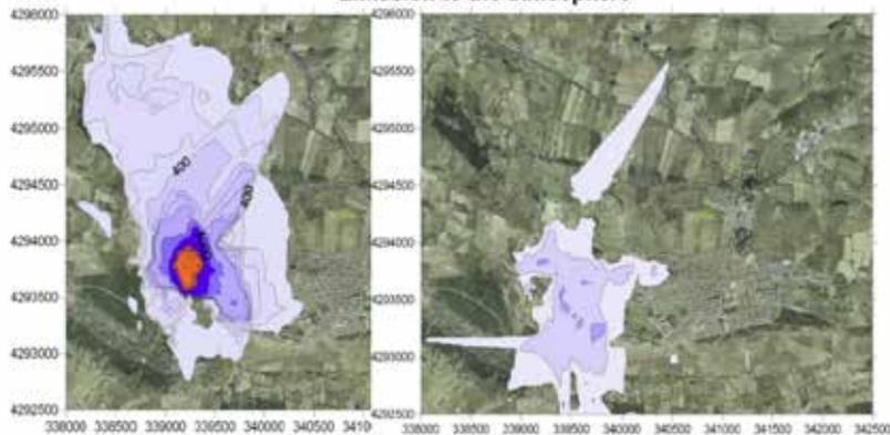
Test in the air during the works (ng/m3)
