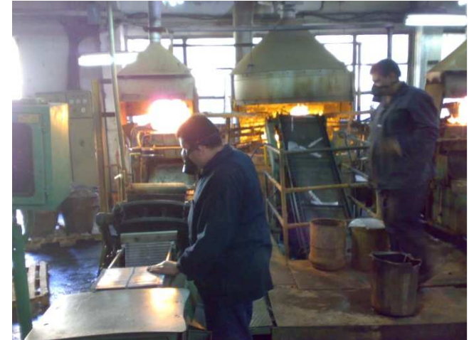
Lead vapor and dust control at Egyptian Plastics, Alexandria
