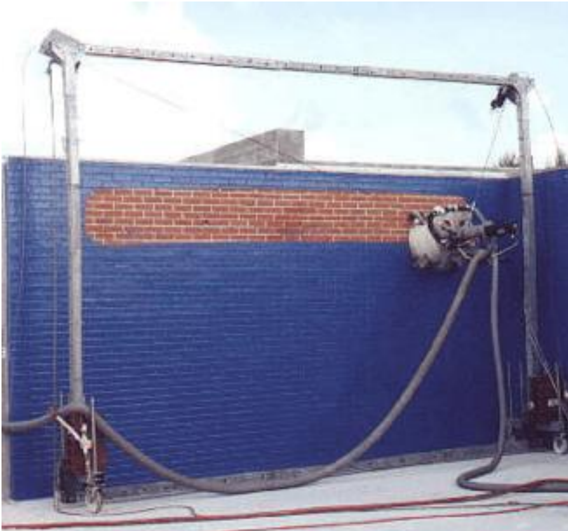
Figure 6 Equipment for removing PCB-containing paint (picture: Pentek USA).
