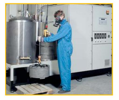
Fluorescent podwers from lamps and other waste containing mercury such as button cells, dental amalgam are placed in the vacuum chamber of the distiller.
