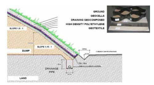
SEALING SURFACE SCHEME High inclination slope C) installation of a water collection, circulation and discharge system This stage of the remediation aims to prevent erosion that may affect the stability of the slag heap. A water collection, circulation and discharge system was installed, through the construction of ditches, drainpipes and perimeter channels that collect runoff and prevent future erosion, which would affect the stability of the slopes.
