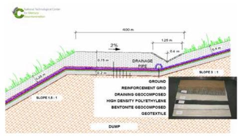
SEALING SURFACE SCHEME Low inclination slope
